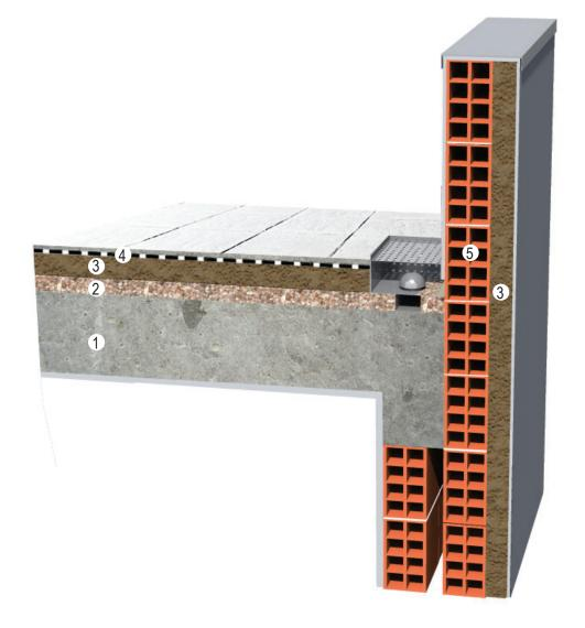
The support must be executed with 1% to 2% slope. The waterproofing must prevent the passage of water into the interior, ensuring that the singular points (connection to parapets, chimneys,...) are planned with special attention. When asphaltic membranes are used, a geotextile shall be applied between them and the insulation layer.
