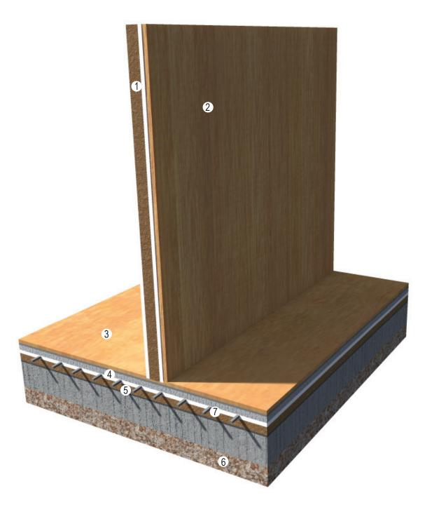
Natural insulation is the ideal choice, as it is from renewable origin and has great potential for reuse and / or recycling. The interior wall solution presented consists of a light partition made of laminated plaster board, with expanded cork agglomerate insulation inside.
