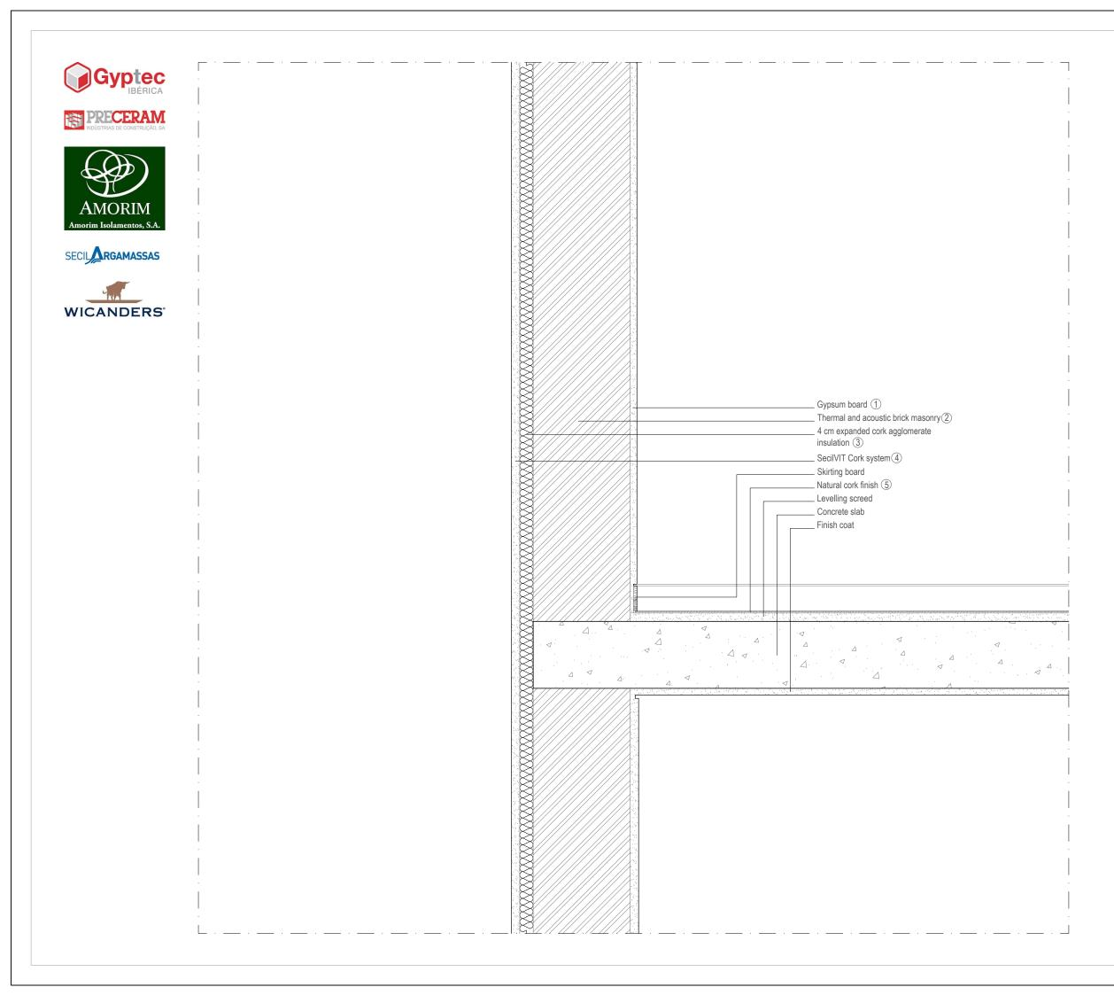
The thermal and acoustic brick differs from the traditional one on its geometry and insulation features.
